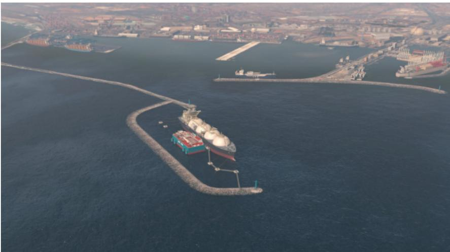
*An impression of the new breakwater, which will provide protection for the permanently sited floating regasification unit, storage vessel and visiting LNG carriers Photo: Gasfin*
